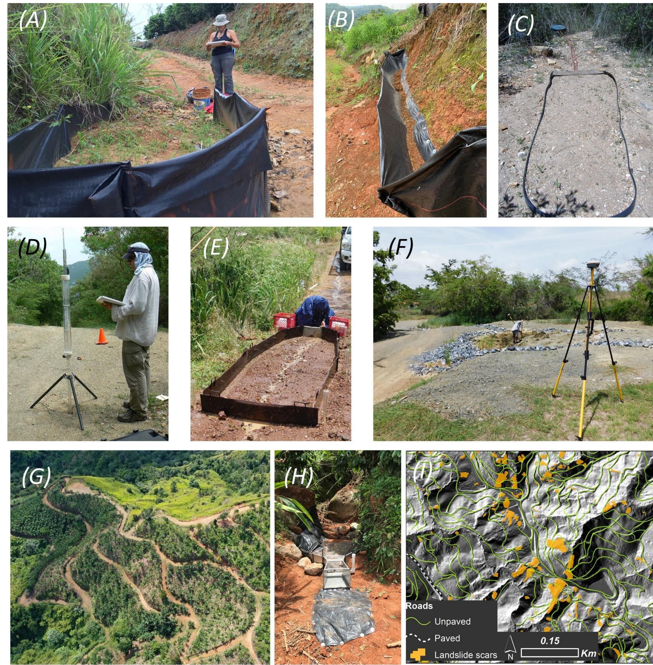
Methods: (A & B) Sed. traps; (C) Runoff plot; (D) Guelph; (E) Rain simulations; (F) Det. pond survey; (G) GIS mapping; (H) Flumes; (I) Landslide mapping & repeated lidar digital elevation model analyses
