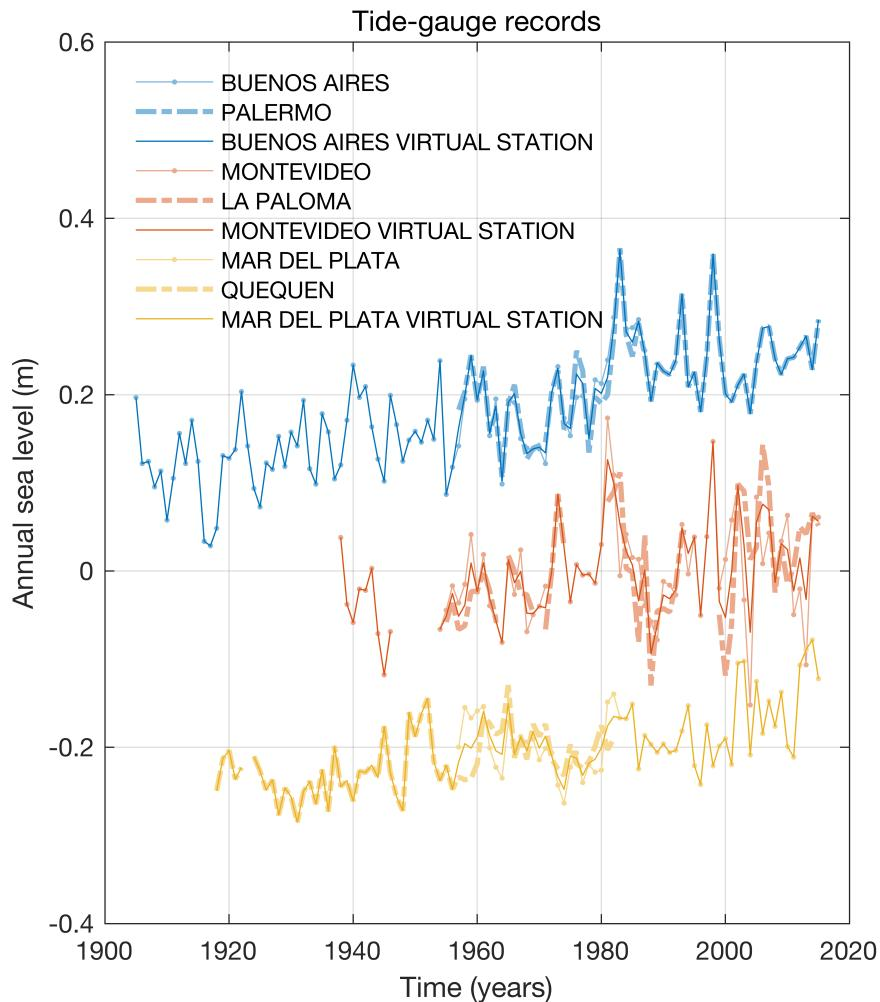
131 FIG. 4. Yearly tide-gauge relative sea-level records (Figure 1, Table 2). Virtual-station time series are shown
