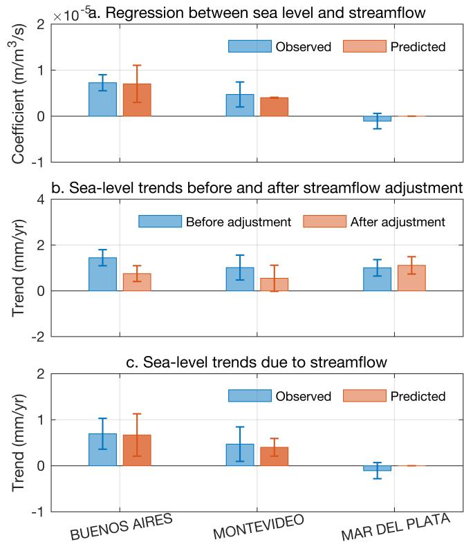
203 FIG. 7. **(a.)** Regression coefficients between sea level and streamflow found empirically from linear regression
