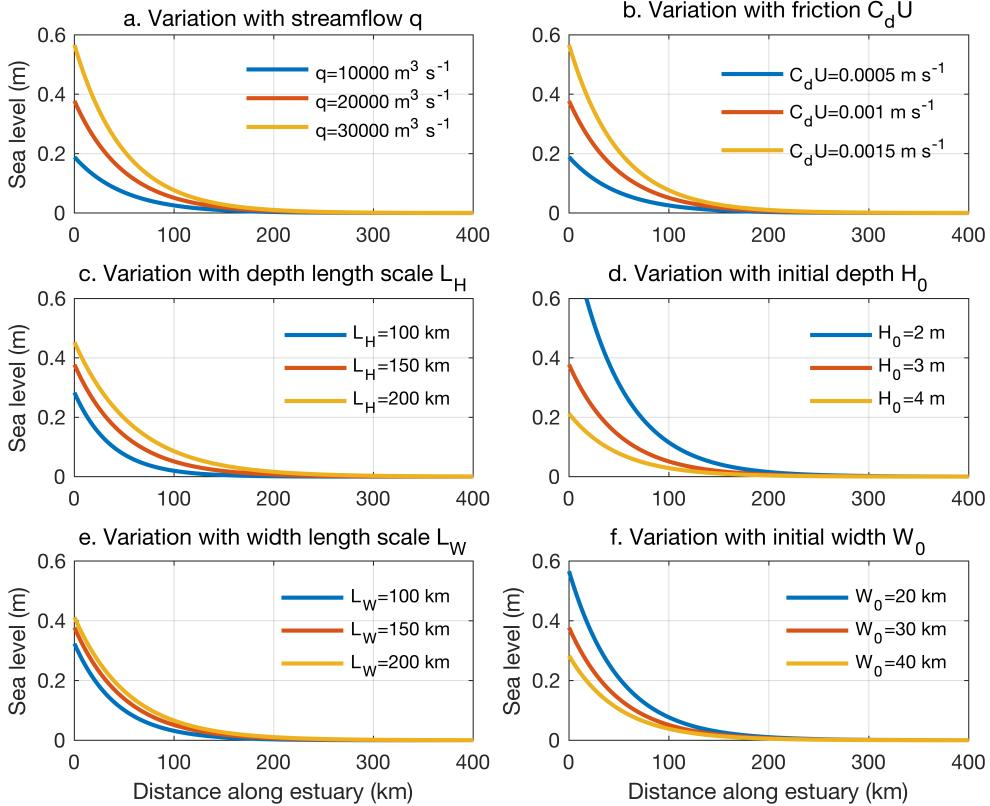
245 FIG. 8. Sea-level response  $\langle \zeta \rangle$  to streamflow forcing  $q$  described by Equation (12) as a function of distance
