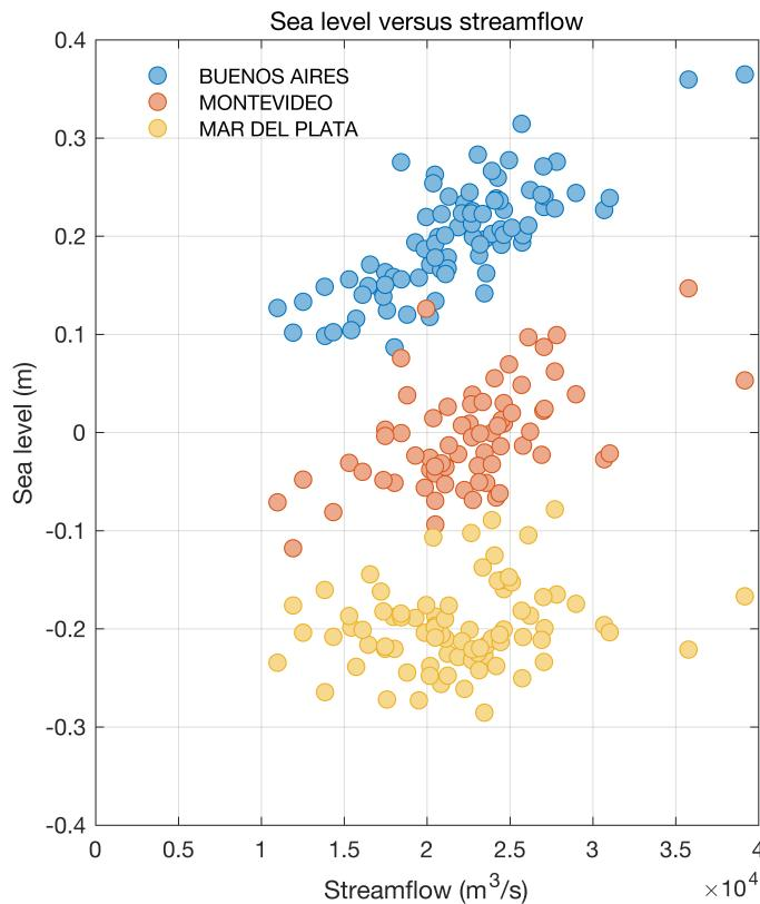
182 FIG. 6. Scatter plots comparing yearly average Río de la Plata streamflow (horizontal axes) and relative sea
