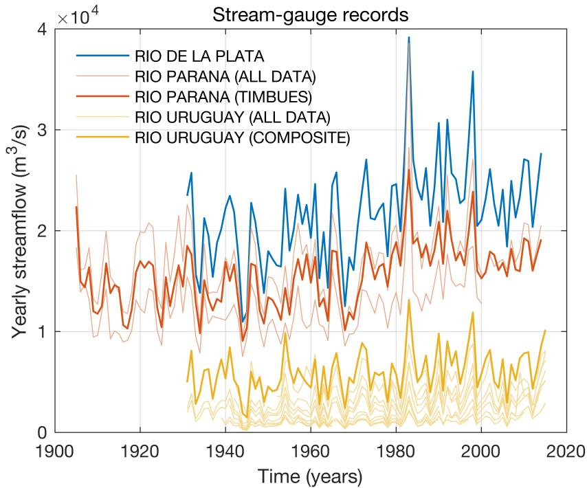
112 FIG. 3. Yearly river-gauge streamflow records (Table 1). The thick black Río de la Plata time series is the sum
