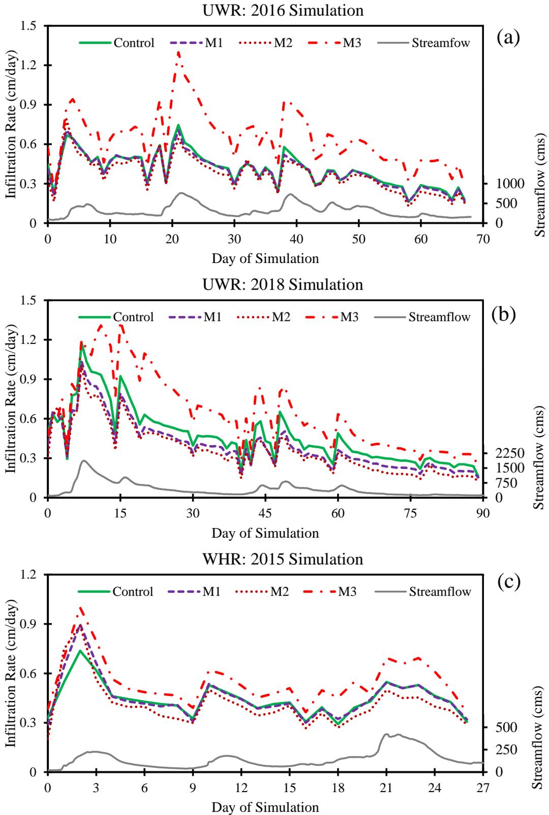
**Figure 11:** Daily infiltration rate in the floodplains of UWR for (a) 2016 simulation, (b) 2018 simulation and (c) WHR for 2015 simulation. The observed outlet hydrograph is shown in grey line on secondary axis.
