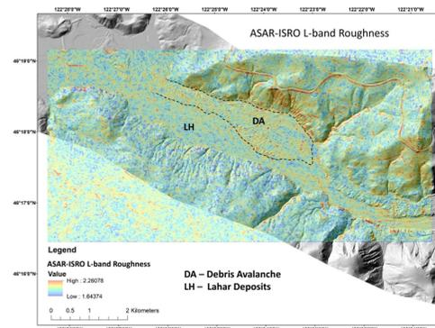
Figure 5. ASAR-ISRO L-band Roughness map (derived from backscatter), superimposed on a 3-m Lidar DEM of Mt St Helens (USGS).
