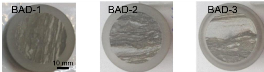
Figure 5. Photographs of the three heterogeneous drill core samples (BAD1 – BAD3) used in the HTO-through diffusion experiments. Dark grey: clay-rich layers, light grey: sandy layers containing quartz and carbonates (mainly calcite) in different proportions.
