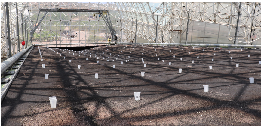
Figure 1. Center hillslope with cups to measure the rainfall distribution. The picture is taken at the upslope end looking downslope.
