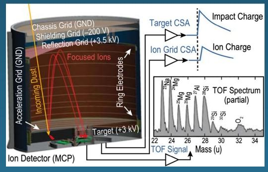
Functional drawing of IMAP's dust detector (IDEX) which will allow measurement of dust composition. ISP's detector should have such capabilities (from McComas et al. (2018))
