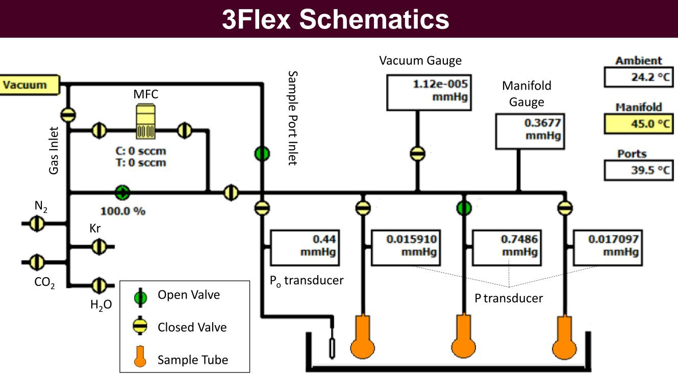
▲ The operation of 3Flex is governed by automated control of 15 solenoid valves, 1 MFC, 1 vacuum pump unit, 2 pressure gauges, and 4 pressure transducers for 3 sample tubes in a dewar cooler.
