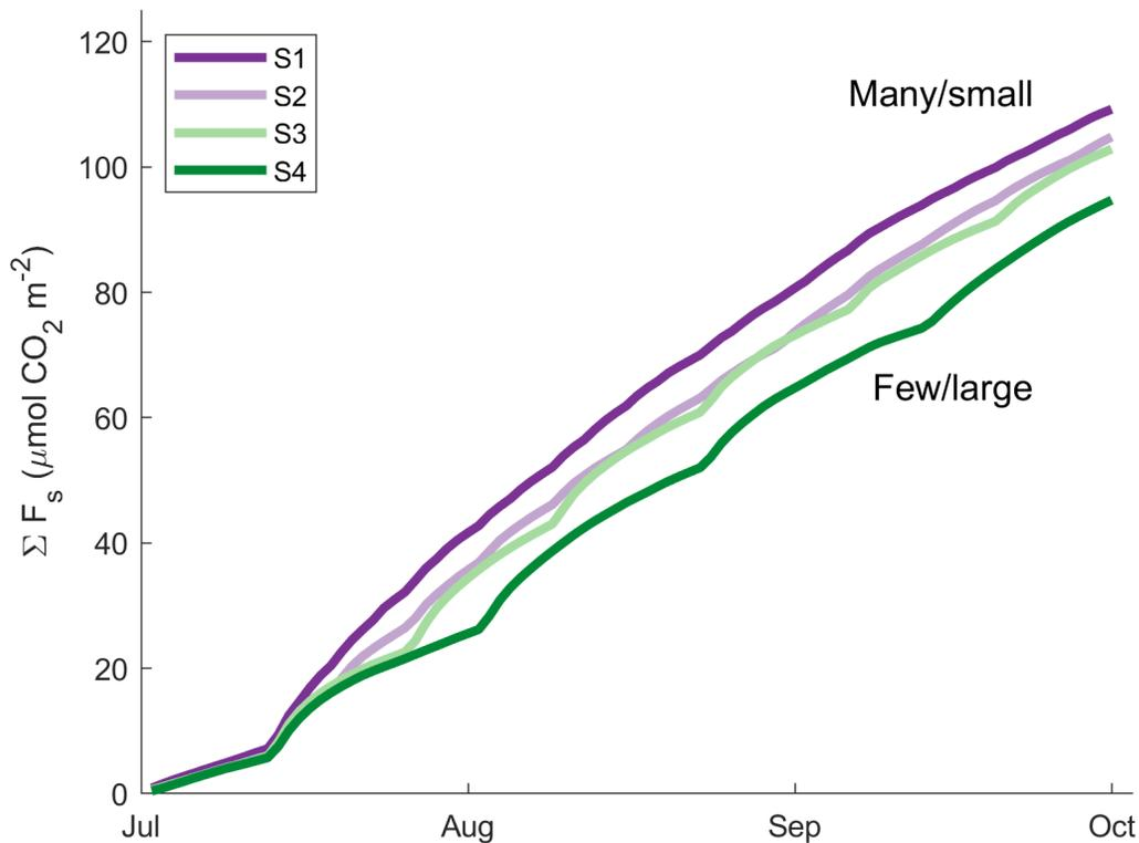
Figure 9. Cumulative daily soil CO<sub>2</sub> efflux (F<sub>s</sub>) under four levels of rainfall repackaging during the summer 2020 growing season. S1 to S4 are a gradient from many/small to few/large rainfall events.
