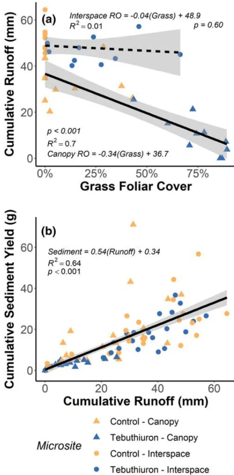
Figure 12. Regression of grass foliar cover and run-off by microsite during fine-scale (0.5 m) 120 mm h<sup>-1</sup> intensity rainfall simulations (a). Regression of cumulative run-off and cumulative sediment yield at all rainfall intensities (b). Gray bands denote 95% confidence interval.
