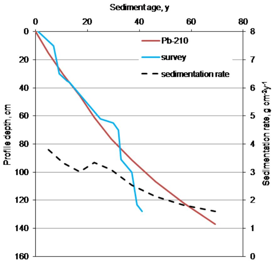
Figure 16. Comparison of sediment age in pond 208 between direct survey measurements and the <sup>210</sup>Pb method.
