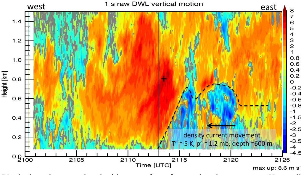
Vertical motion associated with a gust front from a thunderstorm over Huntsville on 30 Aug 2013. The maximum updraft of 8.6 m/s is near 800 m AGL, labeled with "+". The time vs. height section can be viewed as a vertical section in the E-W plane (east on the right) The dashed line shows the inferred structure of the boundary based on vertical motion and radiometer measurements.
