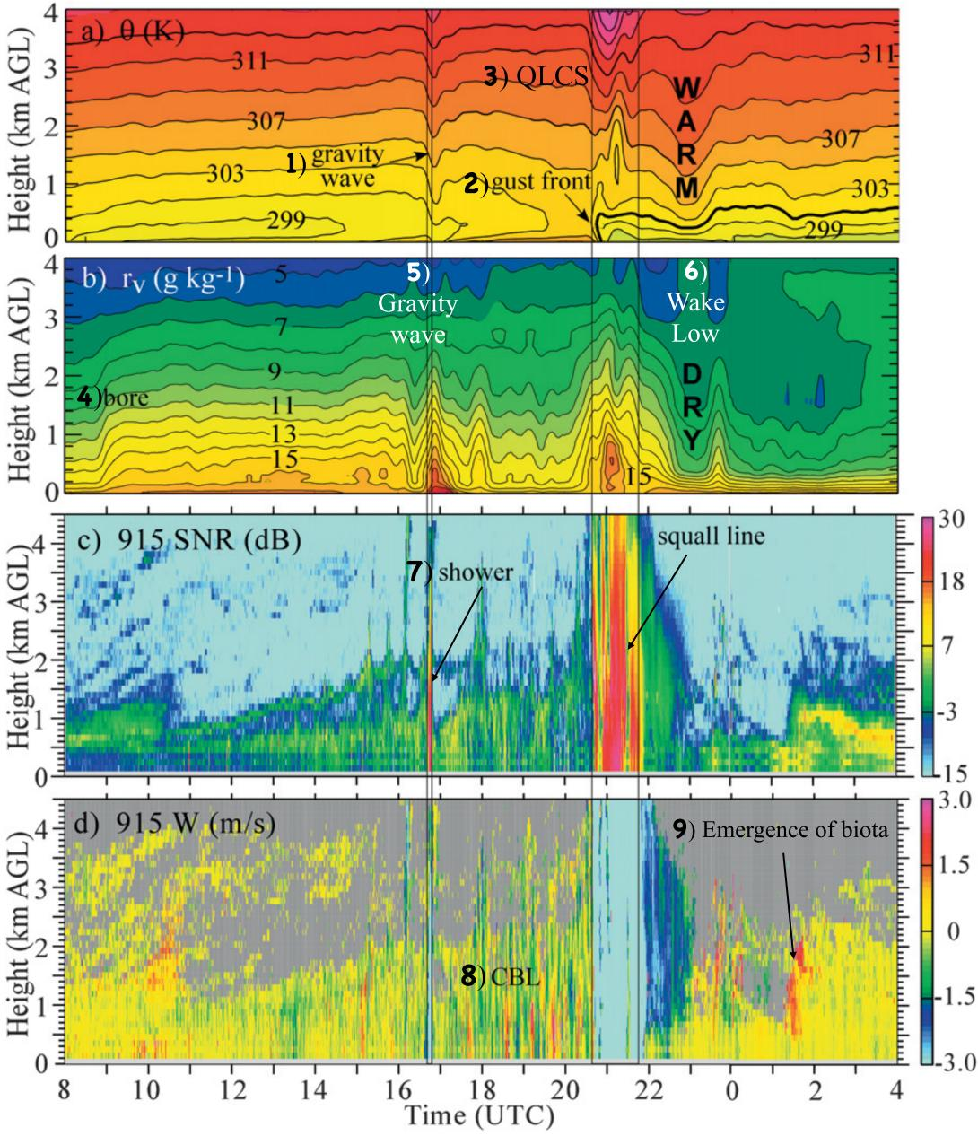
Illustration of features detected by MIPS measurements (based on radiometer (panels a and b) and 915 MHz profiler (panels c and d) on 8 Jun 2007. Ceilometer backscatter and surface measurements are not shown. Features are annotated and labeled with bold numbers, 1-9. Adapted from Knupp et al. (2009).
