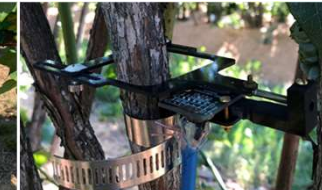
Figure 12: Dendrometer installed on a blueberry plant ( Vaccinium sect. Cyanococcus ) at Lewis-Brown (LB) Farm in Corvallis, OR. We have validated all our devices and conducted various tests at LB Farm since May 2021.
