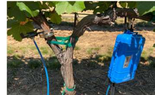
Figure 11: Dendrometer installed on a grapevine ( Vitis vinifera L.) at Southern Oregon Research and Extension Center (SOREC) in Central Point, OR. Seventeen devices were deployed for 6-12 weeks during summer 2021. The devices were deployed on plots receiving two different water treatments.
