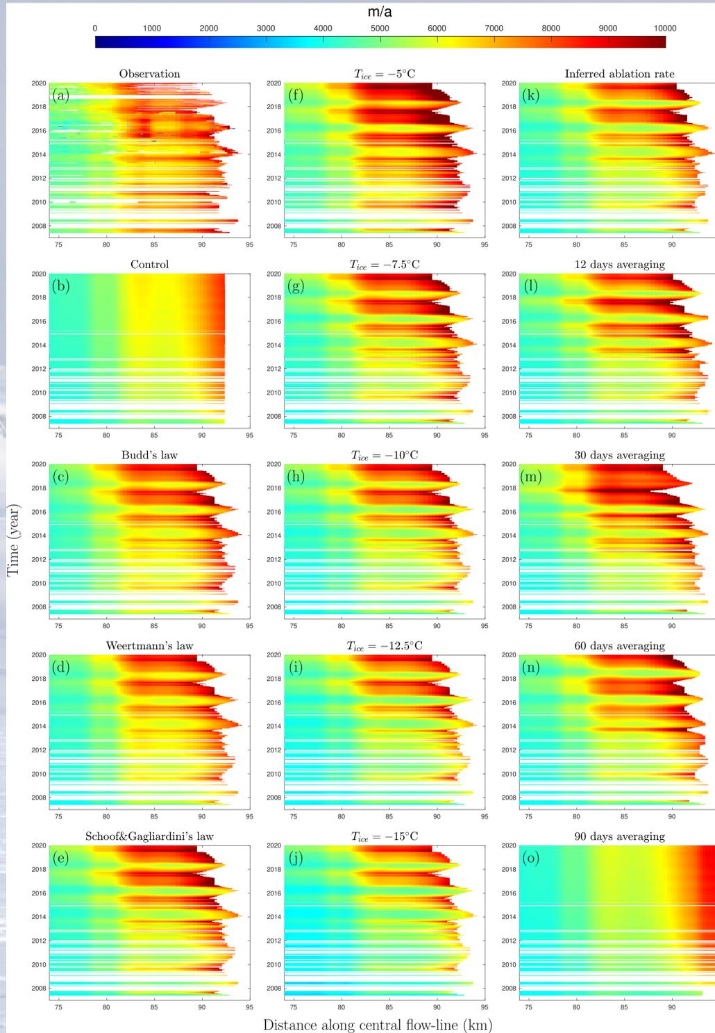
Figure 3: Hovmöller diagram of ice velocity along the central flowline of the (a) observation, (b) control run with fixed calving front position, (c)-(e) different friction laws, (f)-(j) different ice temperatures, (k)-(o) use inferred ablation rate. The x-axis indicates the distance along the flowline and the y-axis is time.
