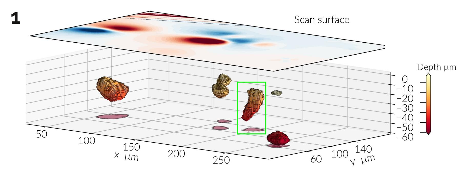
In **FIG 1** a scan surface records the out of plane magnetic field signal from the individual grains. In this case we show the results of scanning SQUID magnetometry applied to a synthetic sample with magnetite grains, which is reported in [2]. Below this surface the profiles of the magnetic grains are depicted as aggregations of cuboids. These profiles are modelled from micro-CT measurements, which also provide the location of the particles.
