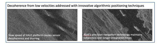
**SWaP Constraints:** Aloft's positioning techniques rely on computational processing and significantly relax the requirements on IMU support hardware, providing a path towards lower overall system size, weight, and cost. To further reduce SWaP, without compromising on performance, Aloft leverages advances in off-the-shelf radio-frequency integrated circuit (RFIC) and System-on-Chip (SoC) hardware technology to create a tightly-integrated, high-performance, and affordable payload solution.
