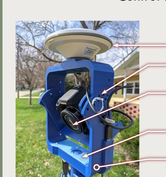
Dual-freq GNSS Adjustable Tilt Customizable Camera Cradle Inertial Measurement Unit (IMU)
