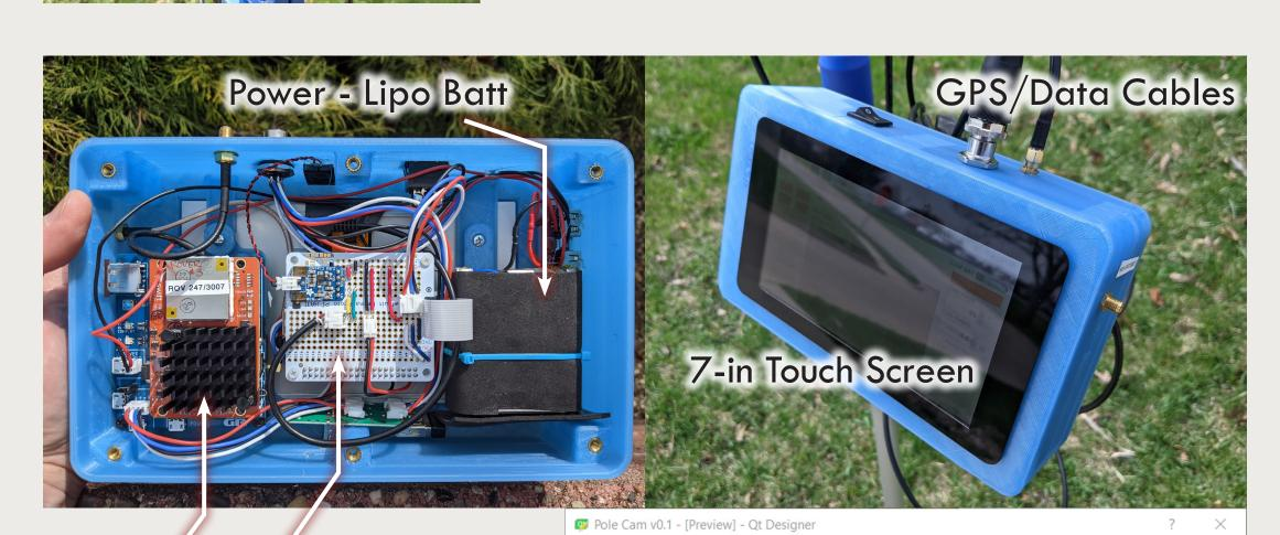
Swiftnav Raspberry Pi 3a, Piksi Multi Screen Controller, Data Connections
