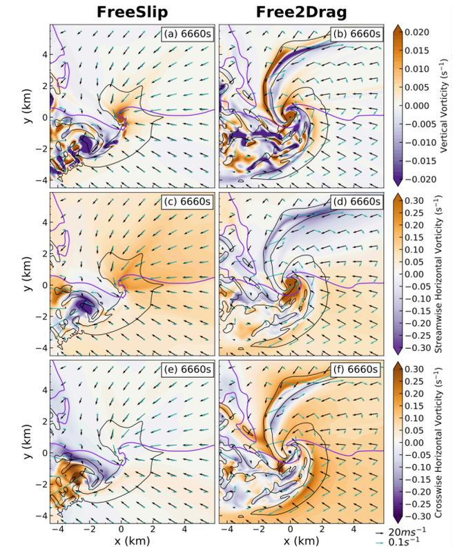
**Fig. 6.** Distribution (shaded) at 30 m AGL of vertical (top row), horizontal streamwise (middle row), and horizontal crosswise (bottom row) vorticity (shaded). Radar reflectivity (purple contour), storm-relative horizontal wind (black arrows) and horizontal vorticity vector (Green arrows) are also shown.
