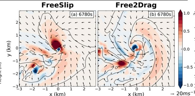
**Fig. 5.** vertical acceleration at 200 m AGL (shaded).
