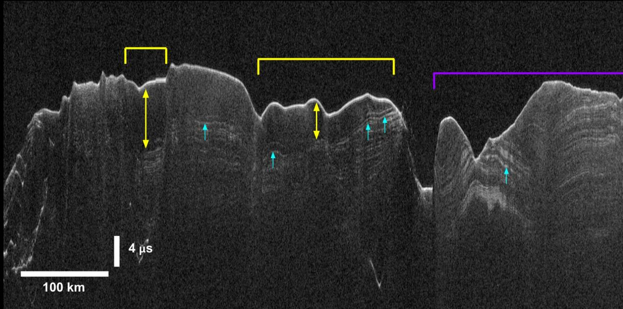
Light blue arrows point at subsurface radar reflectors.
