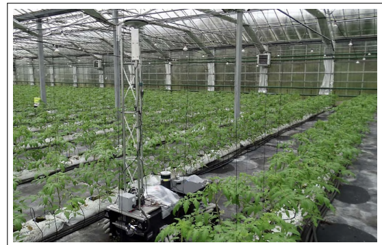
Fig. 4. Autonomous telemetry system for data collection using high precision GNSS geolocationing system by M. Pattinson et al. [11]
