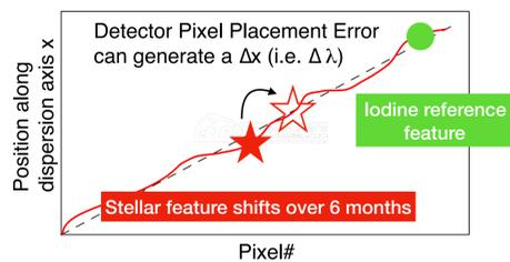
6 month Earth orbital velocity change causes different pixels to be used, which can cause different  $\Delta x$  error
