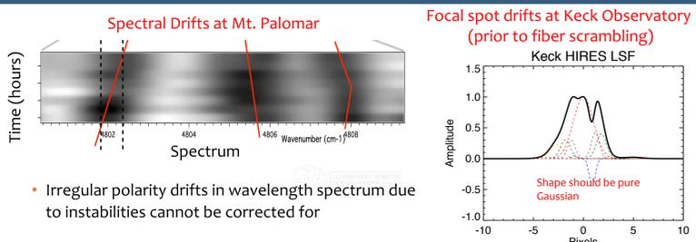
Irregular polarity drifts in wavelength spectrum due to instabilities cannot be corrected for
