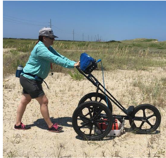
Geophysical Survey Systems, Inc. (GSSI) SIR 3000 GPR, 400 MHz antenna
