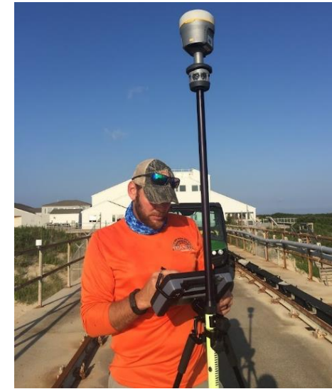
Trimble R10 Global Navigation Satellite System (GNSS) receiver + NC Geodetic Survey's Real Time GNSS Network
