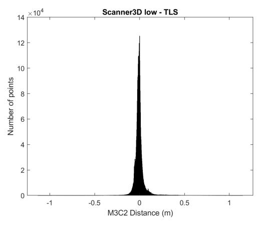
Mean M3C2 distance: -0.0017 m MAE M3C2 distance: 0.037 m Std. Deviation M3C2 distance: 0.083 m
