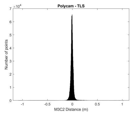
Mean M3C2 distance: -0.0057 m MAE M3C2 distance: 0.028 m Std. Deviation M3C2 distance: 0.075 m
