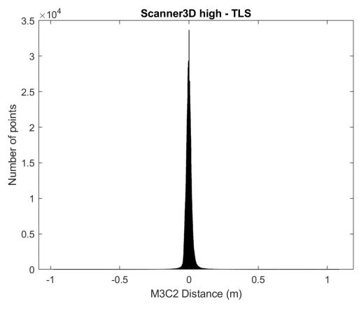
Mean M3C2 distance: 8.5e-05 m MAE M3C2 distance: 0.018 m Std. Deviation M3C2 distance: 0.039 m
