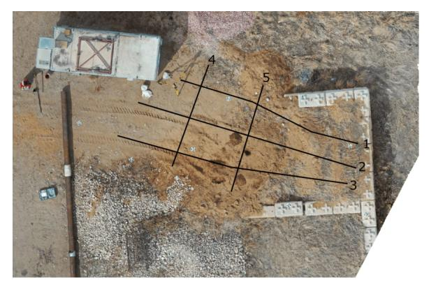
Each extracted profile was compared to the TLS profile, and the mean absolute error of the each profile relative to TLS was computed.
