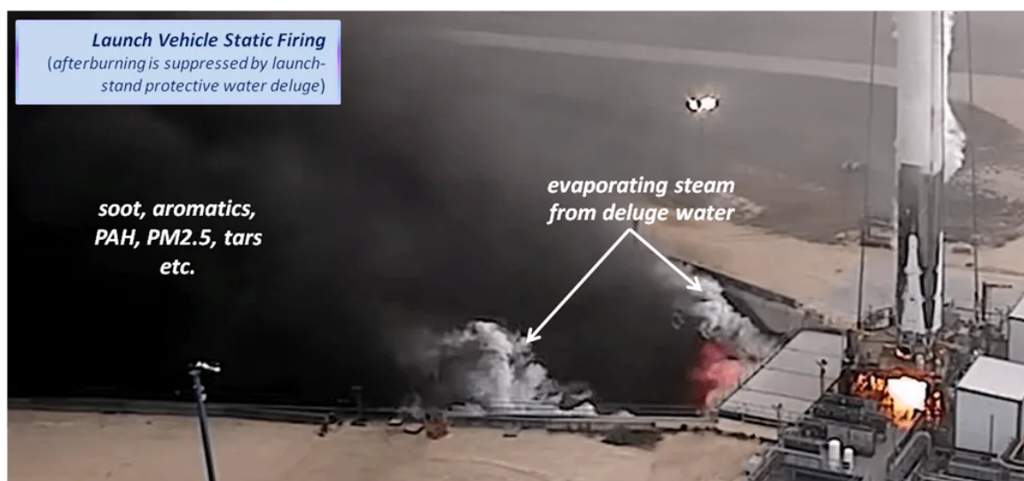
Figure 4. Static firing - deluge water below vehicle prevents facility damage by the hot plume - but deluge water also shuts-down tropospheric afterburning of the soot, aromatics, PAH, tars, etc. created by the gas generator and film coolant flows, which then form the large dark cloud (PM2.5, PAH, aromatics, etc., left). [ref. C]
