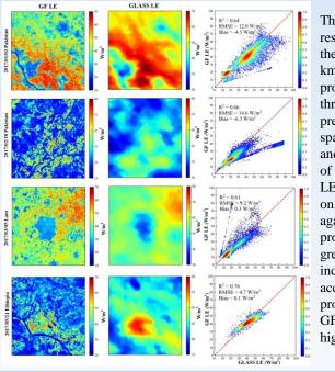
The validation results show that the 16 m GF and 1 km GLASS LE products of the three countries all presented good spatial consistency, and the coefficient of determination of LE estimates based on GF-1 data against GLASS LE products were all greater than 0.6, indicating that the accuracy of LE products based on GF-1 data was high.
