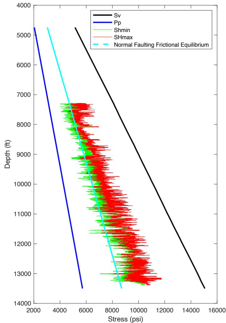
Figure 3: The stress profile obtained from the integrated earth model.
