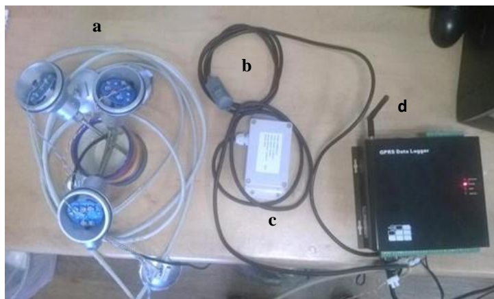
Figure 6. The monitoring system components: (a) high temperature sensors; (b) humidity and air temperature sensor; (c) CO 2 concentration sensor; and (d) data collecting device.
