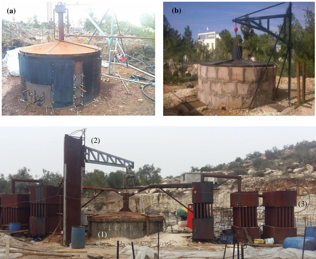
Figure 2. The prototypes that were built at Ariel University: (a) Prototype 1 (capacity 100-200 kg of wood) and (b) Prototype 2 (capacity 1000-2000 kg of wood). The third ERS prototype (c) was built and operated at the Ya'bad site in the Jenin area. The system's structure consists of: (1) the body of the kiln; (2) the hoist for lifting and lowering the lid; (3) the condenser system for gas absorption.
