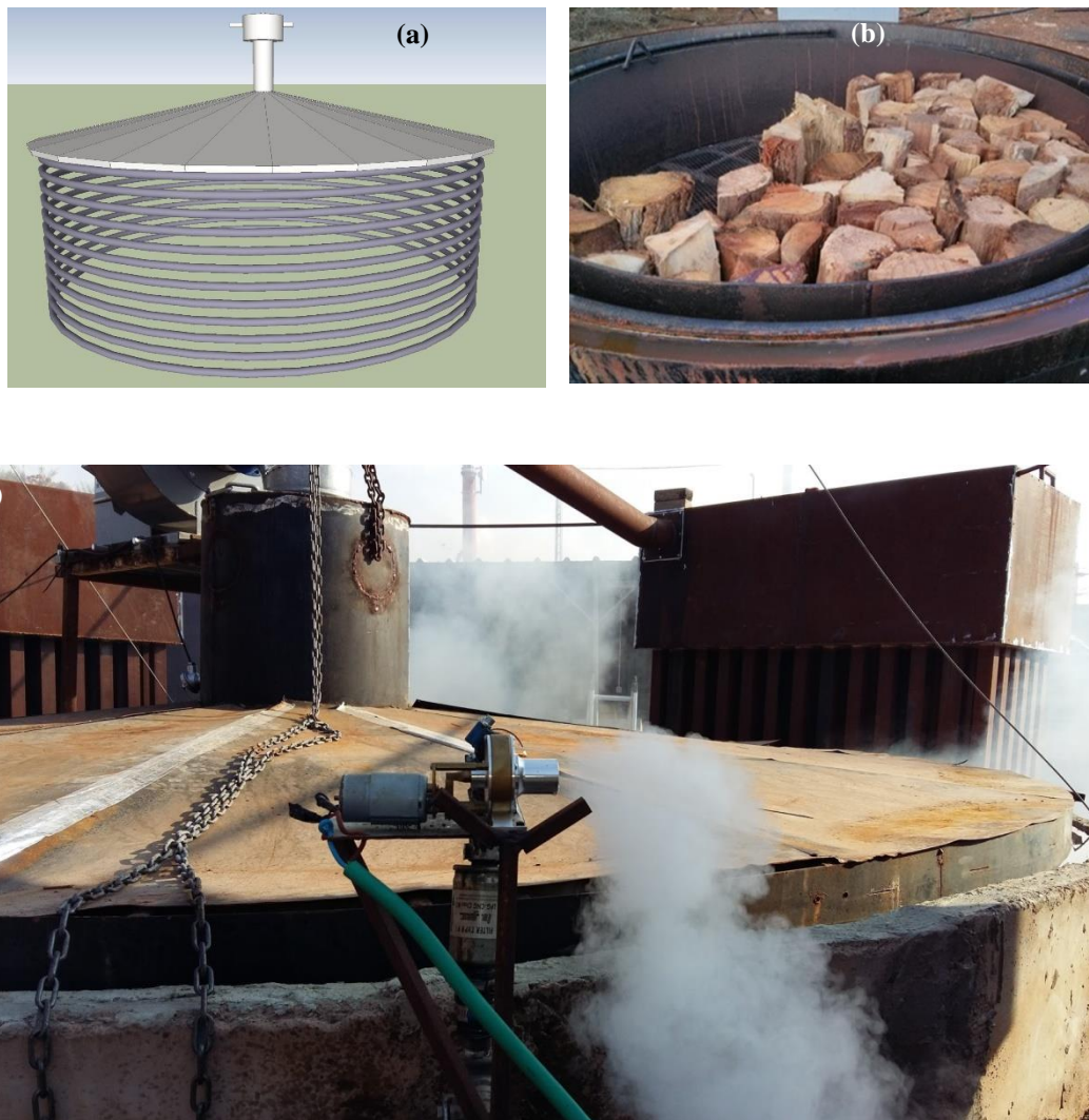
Figure 3. Cooling pipe systems (a) heat converter illustration; (b) Ariel University pilot with wood arrangement in the pyrolysis chamber and (c) the steam turbine operation at the Ariel pilot.
