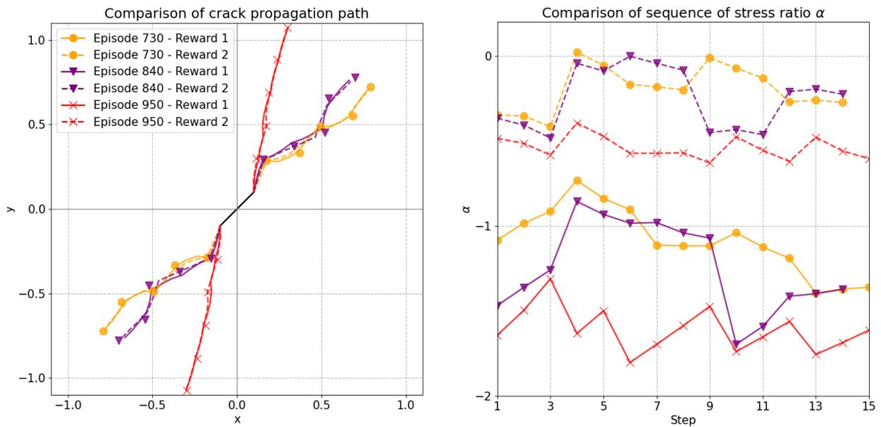
**Figure A1.** Comparison of crack path and sequence of stress ratio  $\alpha$  using reward function 1 and 2.
