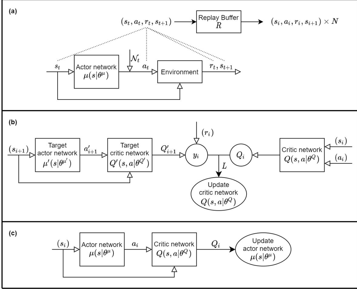
**Figure 1.** Illustration of the DDPG algorithm developed by **Lillicrap et al. (2015)** that is adapted and modified for the proposed reinforcement-learning-based control of mechanical discontinuity. (a) The interaction between the RL agent and environment and the use of replay buffer. (b) The procedure for updating the critic network. (c) The procedure for updating the actor network. In the subplots (b) and (c), the parameter in the bracket indicates that it is sampled from the replay buffer.
