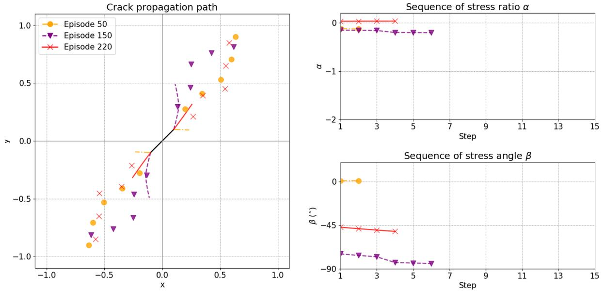
**Figure 8.** The crack propagation paths (left) and corresponding actions (right) taken by the RL agent at randomly selected early stages of training (episodes 50, 150 and 220). RL agent uses reward function 2 for the desired control. RL agent during early learning episodes is not able to take actions to perfectly track the predefined crack path. The early performance using reward function 2 is worse than the reward function 1.
