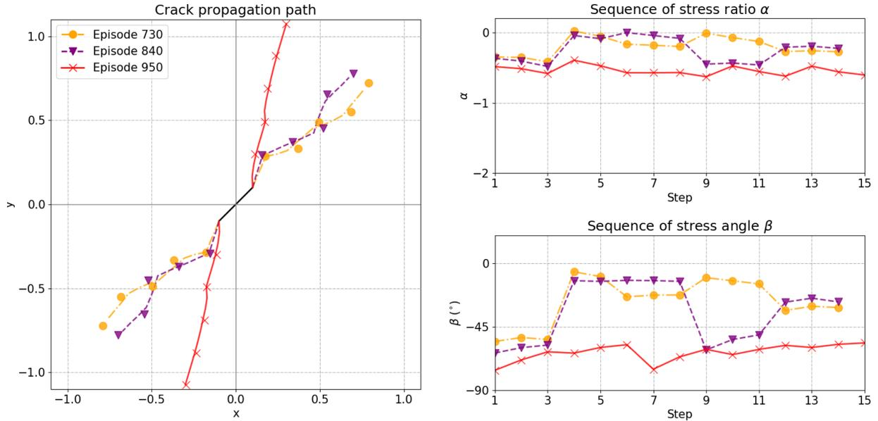
**Figure 9.** The crack propagation paths (left) and corresponding actions (right) taken by the RL agent at randomly selected early stages of training (episodes 730, 840 and 950). RL agent uses reward function 2 for the desired control. RL agent during late learning episodes is able to take actions that result in perfect tracking of the predefined crack path.
