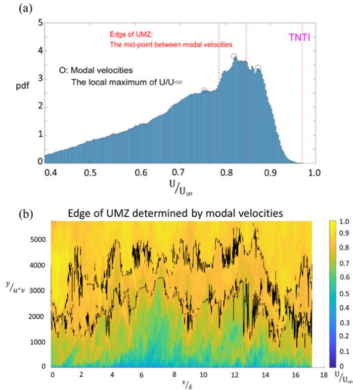
193 **Figure 2.** Illustration of the detection of instantaneous UMZs. (a) The corresponding histogram
