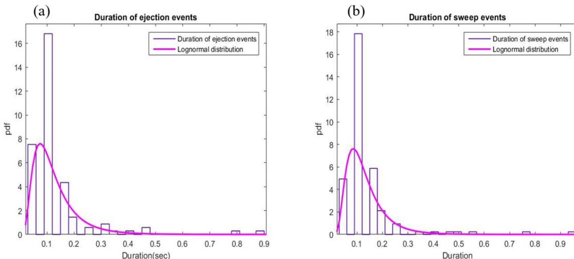
461 **Figure 9.** The probability density function of the duration (lifespan) of (a) ejection and (b)
