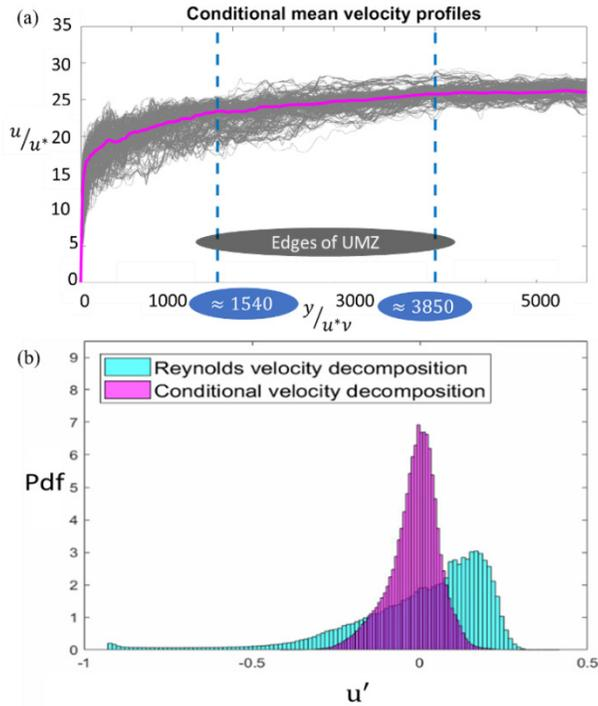
232 **Figure 3.** (a) Conditional mean velocity profiles. (b) Histograms of streamwise velocity
