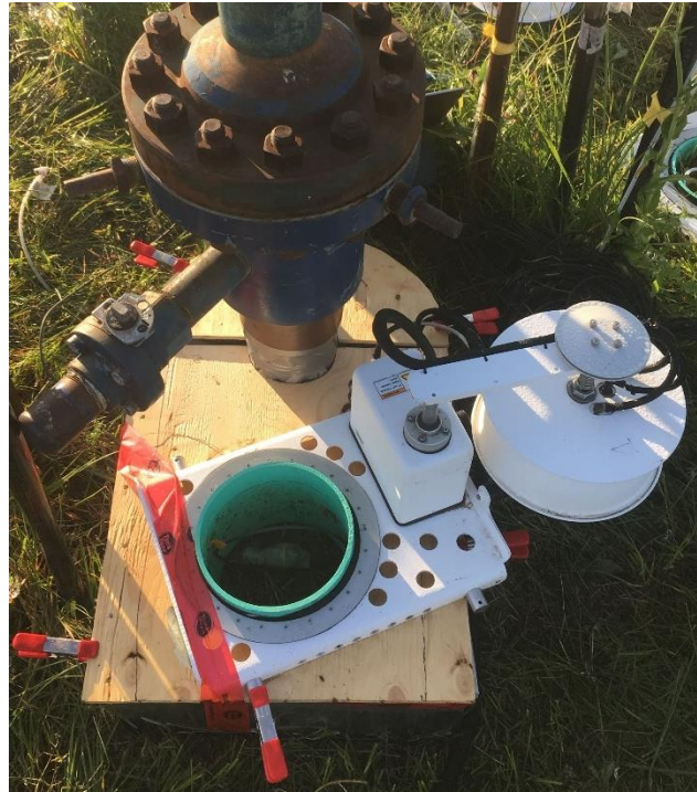
Figure S1 Custom wellhead collar construction schematic and field photograph showing the coupling of the automated dynamic efflux chamber to the custom collar. The collar base was constructed with thin sheet metal placed 2-5 cm into the ground surface around the well (the lateral segment of the surface casing preventing deeper installation). Rigid plastic sheeting formed an air-tight seal on the lid-portion of the chamber. A hole in the plastic sheeting accommodated a 200 mm PVC pipe, allowing for coupling with the automated chamber. A plywood external lid to the chamber provided structural support and prevented any pumping/chamber size modifications due to wind acting on the plastic. Note that the surface casing is vented to the atmosphere outside of the custom collar through a surface casing vent (not shown in schematic).
