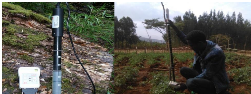
Figure 4: The soil moisture sensor (PR2) and its use in the field
