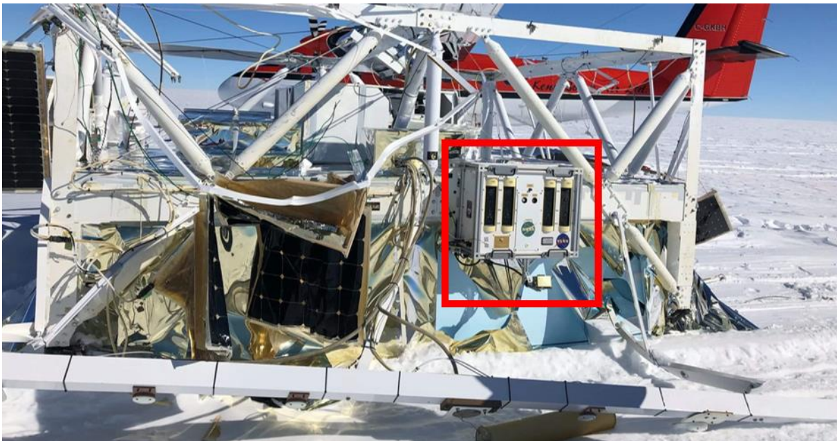
Figure A2. The SuperTIGER-2.3 balloon mission ( red box around the E-MIST payload with the M-42 detector). Picture was taken during the payload recovery operation after landing on the Antarctic ice shelf, following the 32-day mission in the polar stratosphere. © NASA
