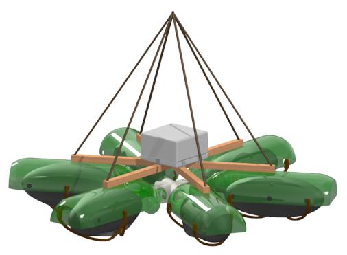
Dropsonde shelters composed of two-litre bottles. Dropsondes are secured by fluorocarbon fishing line (low melting point) and released individually by nichrome hot-wire cut-down mechanisms controlled by the payload electronics.
