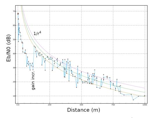
In this figure, dots represent successfully-received data packets with no uncorrectable errors.  $1/r^4$  is the expected for line-of-sight near ground communications. (Performance for an airborne instrument will be much improved with reduced interference and  $1/r^2$  scaling.)
