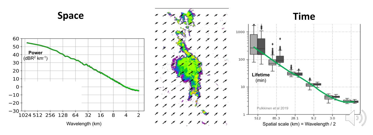
The AR(p) parameters control the rate of evolution at each cascade level consistent with the expected lifetime
