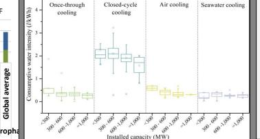
Blue WFs of China's coal fired power plants. The CCP WF is 1.15 l/kWh; WF for closed-cycle cooling is 3-10 times higher than WFs of other technologies. (Zhang, Liu et al., 2017. Journal of Cleaner Production 161: 1171-1179).
