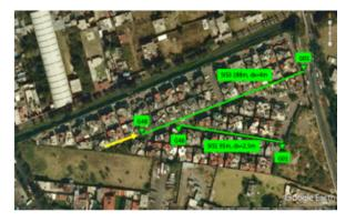
We carry out seismic noise-correlations between all pairs of receivers. The wave trains emerge with amplitude remarkable in time delays less than 2 s. The pulses have a high signal to noise ratio and emerge consistently either in the anti-causal or causal side.
