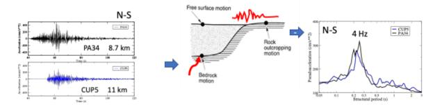
The response spectra of two close accelerometric stations (PA34 and CUP5) show maximum accelerations near 4 Hz (using the 1D VS model indicated by the vertical dashed line).
