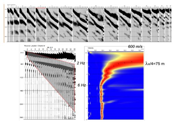
2D Vs sections were built from the interpolation of the 1D Vs profiles. In the first 20 m depth, the dispersion curves do not define the structure; they only indicate a layer with average velocities at 150 m/s. The CMPCC analysis allows defining the Vs lateral variation.
