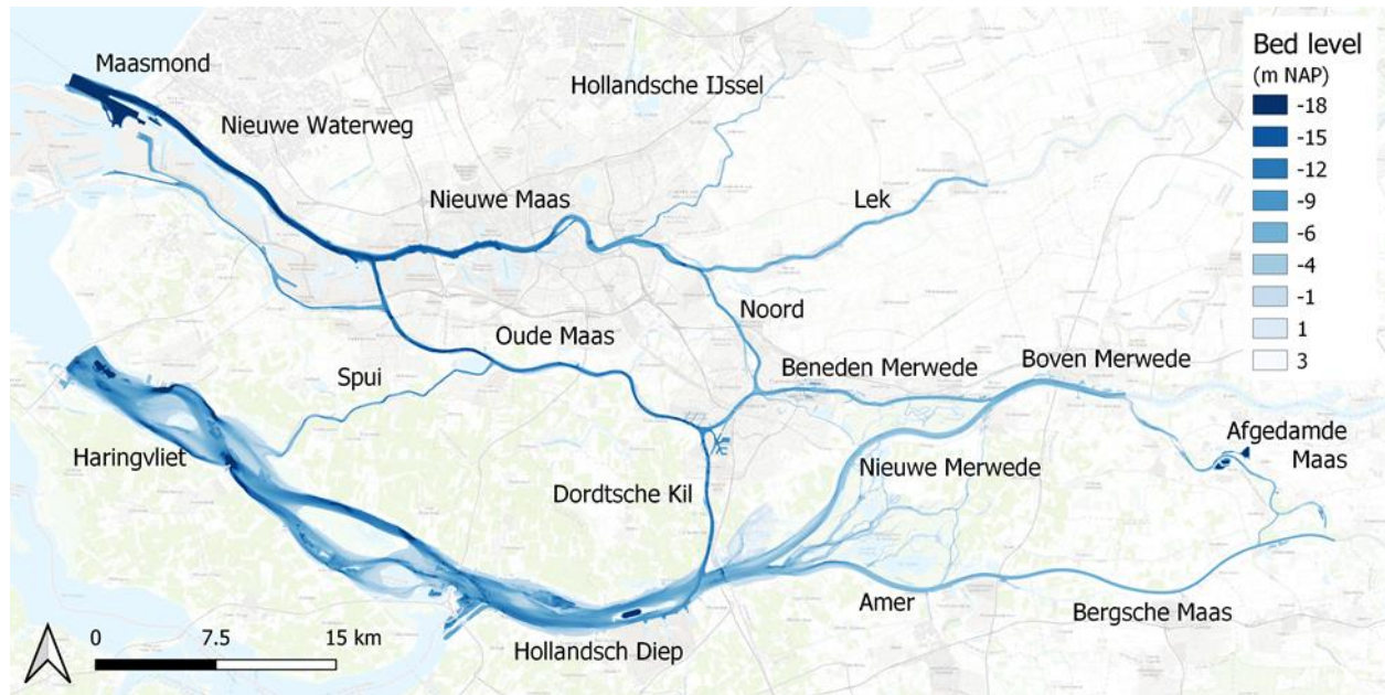
Figure 1 Overview of the river channels forming the Rhine-Meuse Estuary (the Netherlands). In colour the bed level is represented (year 2013, 2014). Map is created in QGIS with the Esri-TOPO base map.
