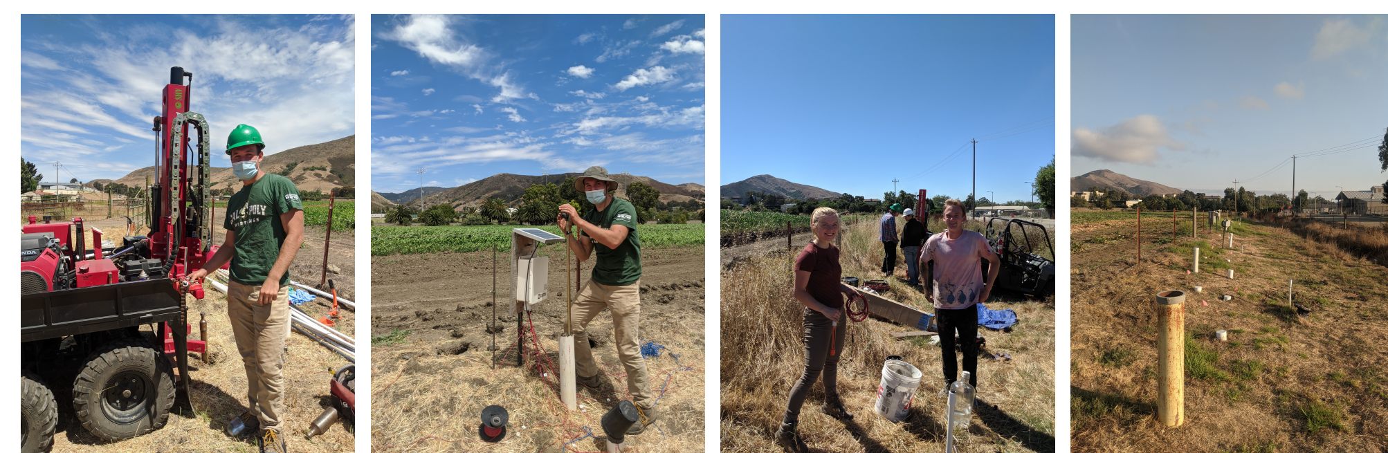
Figure 7: Electrode installation along radial transect. Hand-augured 18 ( d = 3 -in.) holes (2 m intervals) to appropriate depths; Electrodes set in bentonite paste (in dilute CuSO 4(aq) ) at bottom of holes; Conducted 8 constant-rate ( Q = 15 gpm) pumping tests with surface discharge 50 m from well.
