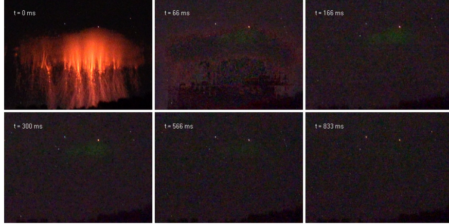
Figure 2. Sprite with green ghost recorded 25 May 2020 at 30 fps (33 ms between mages). The green ghost reaches maximum intensity at t = 166 ms and decays after that. The green in the green ghost images, images 2-6, has been enhanced.
