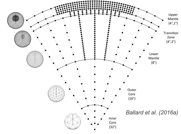
An example of using triangular tessellations of differing resolutions to achieve variable resolution in the radial direction. Points along the radial profiles depict the positions where model parameter values are represented.
