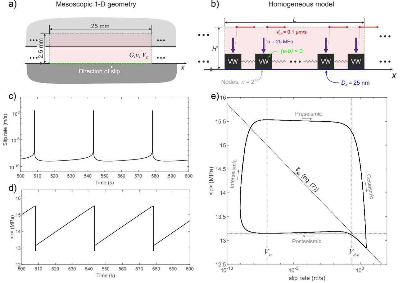
**Figure 5.** (a) General dimensions of the model domain in Figure 1(c). (b) Description of the 1-D boundary value problem being solved by QDYN. RS frictional behavior is described by equations eq5 to eq8. (c) Average slip velocity and (d) average shear stress along the fault for  $t_{sim}$  between 500 to 600s. We see that the fault underwent stick-slip behavior. (e) A diagram of the earthquake cycle for the VW fault that includes preseismic, coseismic, postseismic and interseismic phases.
