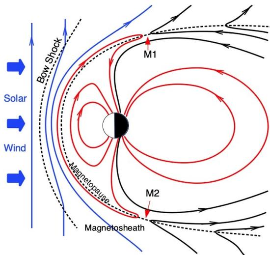
**Figure 1.** Magnetospheric field configuration of magnetosphere for pure northward IMF . Blue and red lines represent IMF field lines and closed field lines, respectively; But a solid black line may be IMF, open, or closed field line. M1 or M2 indicates a magnetic reconnection site. This is a view from the duskside of the magnetosphere.
