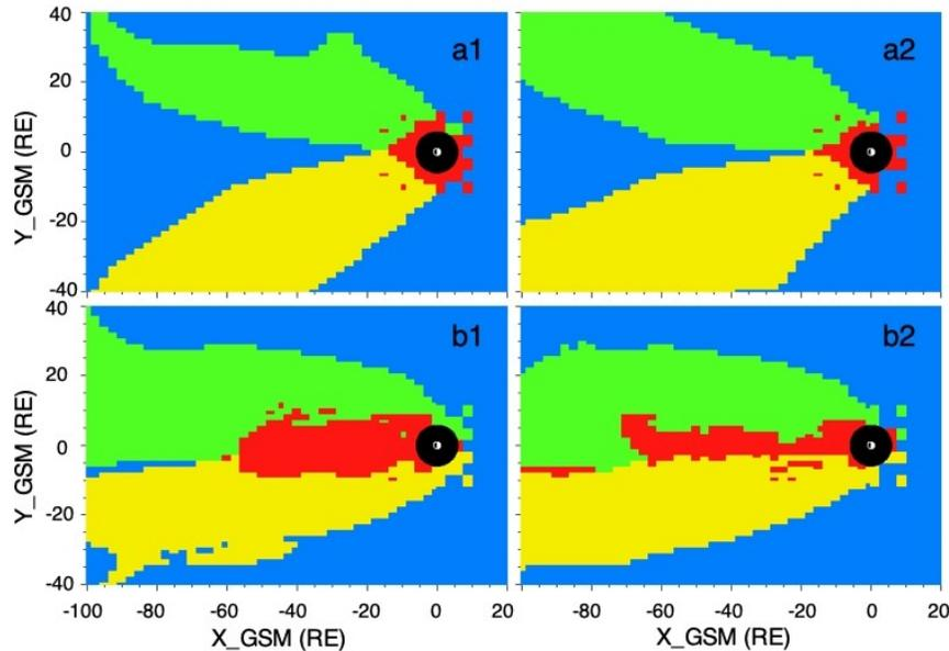
**Figure 5.** Topology distribution of magnetic field lines. The color means the same as Figure 3. The time stamp of (a1) and (b1) is 2000-09-18 00:12:00 UT, and the time stamp of (a2) and (b2) is 2000-09-18 00:30:00 UT. Panels (a1) and (a2) are BATS-R-US simulation results, and panels (b1) and (b2) are OpenGGCM simulation results.
