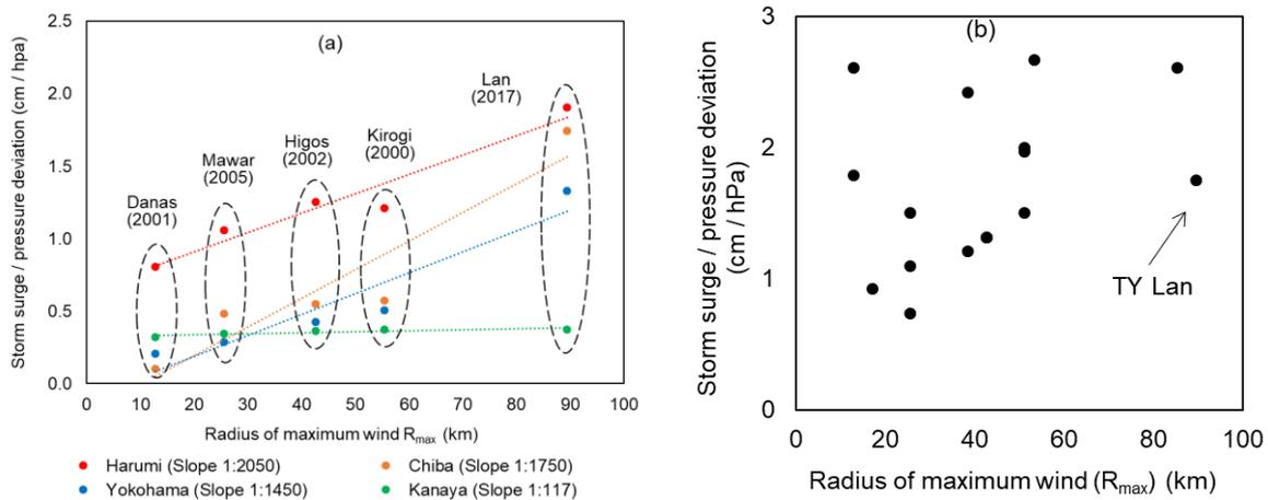
**Figure 3:** (a) Simulated peak storm surge normalized by central pressure deficit vs typhoon size ( $R_{max}$ ) at landfall; (b) Observed peak storm surge normalized by central pressure deficit vs typhoon size ( $R_{max}$ ) at typhoon landfall for Harumi observation station during 1979–2018.
