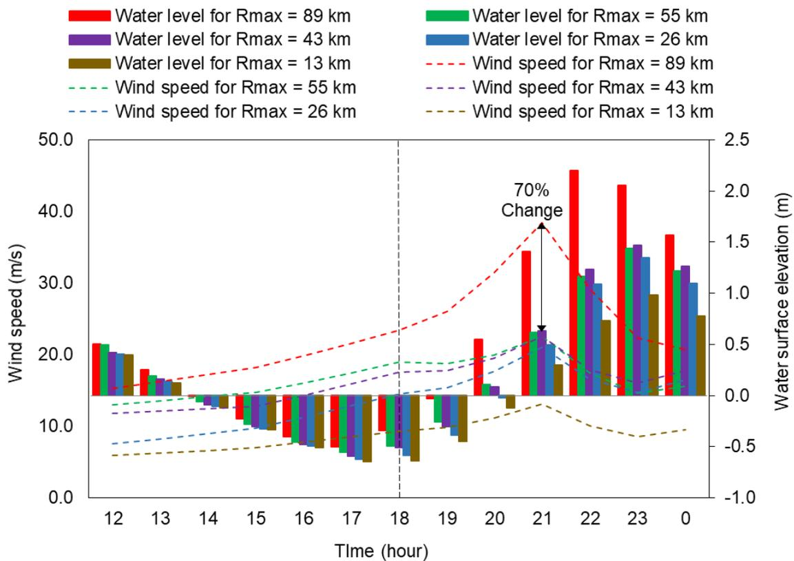
**Figure 4:** Time series (before and after 6 h of typhoon landfall) simulated wind speed and water surface elevation varying with typhoon size at Harumi observation station. The dash black colored line indicates the time of the landfall.
