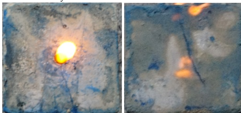
(a) Burning sample with high gas hydrate saturation (from left to right: top view and side view)
