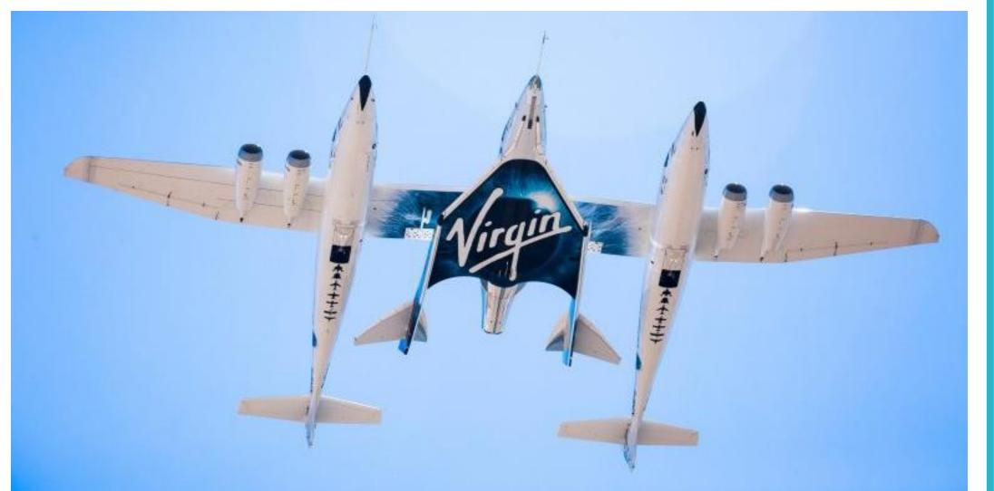
Virgin Galactic use the White Knight Two aircraft from Scaled Composites to carry SpaceShipTwo to its launch altitude. overcome the challenges of developing an aircraft optimised for both ascent and high-altitude cruise.
