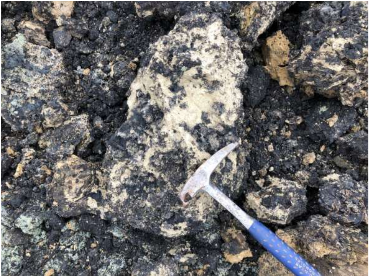
Fig. 5. Oxide-hydroxide ores (black) in mixed oxide-carbonate ore zone
