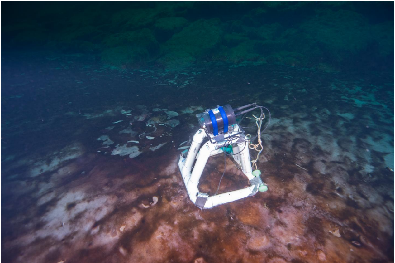
Figure 1. Time-lapse Imaging the sinkhole mat world: Diver image of the deployment position of the time-lapse submersible camera system mounted on top of a PVC frame on microbial mat at the bottom of Middle Island Sinkhole, Lake Huron at ~23 m depth. This diver image was taken around mid-day. Photo credit: Phil Hartmeyer, NOAA Thunder Bay National Marine Sanctuary.
