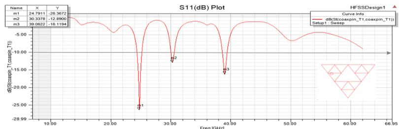
Fig.12. Reflection Coefficient of Sierpinski gasket fractal stage3
