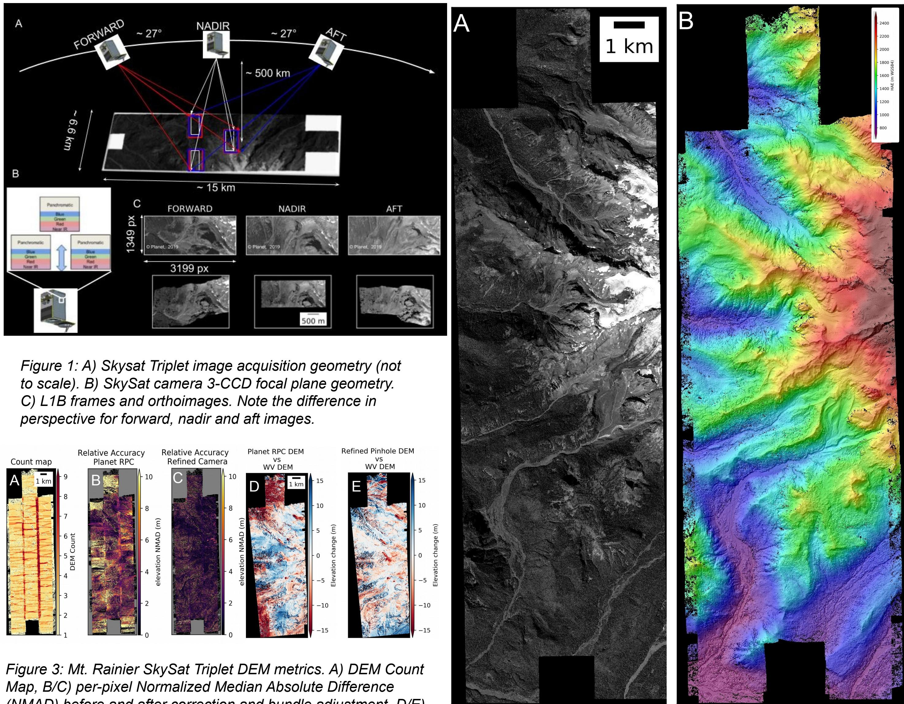
Figure 1: A) Skysat Triplet image acquisition geometry (not to scale). B) Skysat camera 3-CCD focal plane geometry. C) L1B frames and orthoimages. Note the difference in perspective for forward, nadir and aft images.
