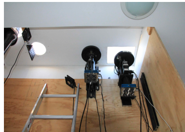
Figure 3. The All-Sky Imagers: ASI-1 is seen at the left of the picture and ASI-2 at its right side.
