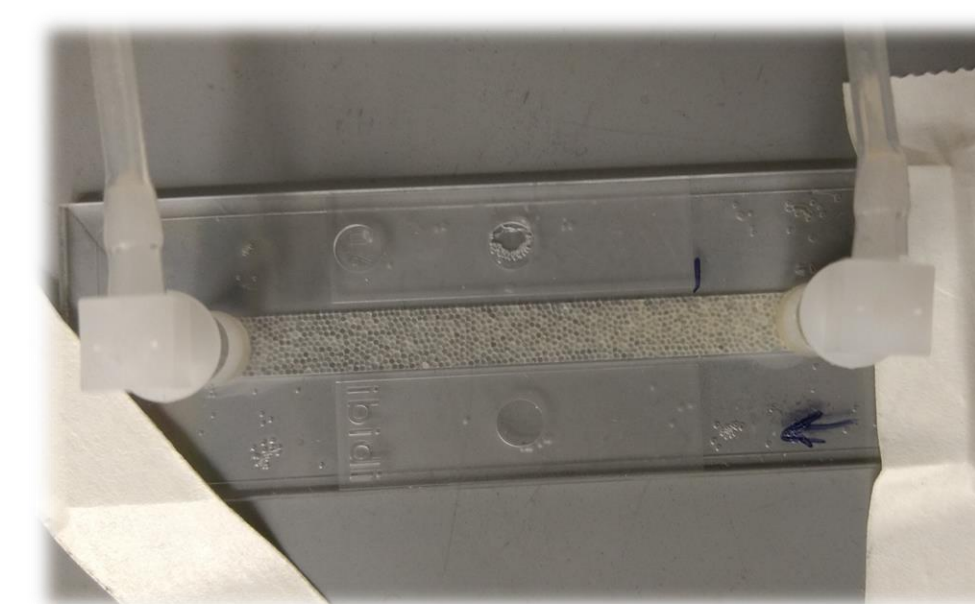
Microfluidic channel ( 50 \times 5 \times 0.6 mm) Packed with 0.5 mm glass beads E. Coli K-12 MG1655 used to form biofilm LB broth used as the feed
