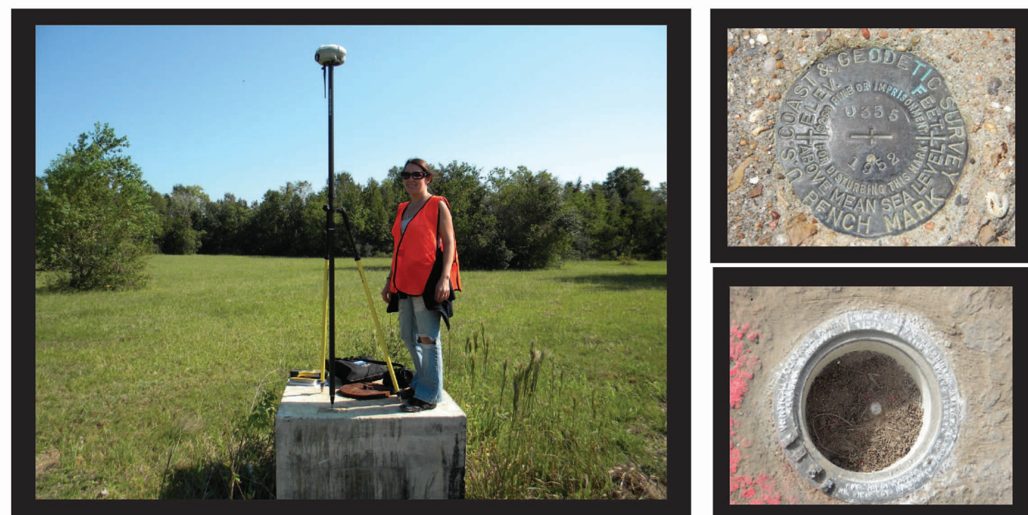
Left: Student measuring a benchmark using the Trimble R8 GNSS GPS. Right: Examples of benchmarks used in survey.
